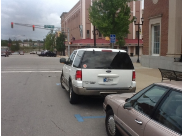
Photo illustrates on-street parallel parking on Main St. Parking space is located near curb ramp and signage is provided in appropriate manner. No access aisle is required.
