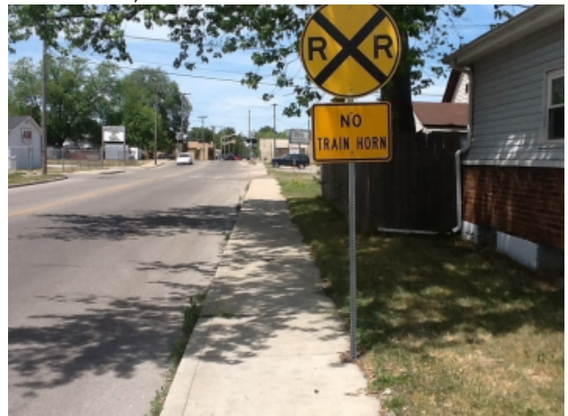
Example of Railroad signage as protruding object within the pedestrian circulation area (Division St. between Marion St. and railroad tracks)
