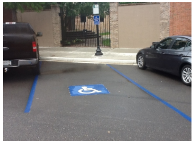
Photo illustrates on-street angled parking with no access aisle provided. Adjacent cars limit width necessary for entry and exit of vehicle. Space also located midblock.
