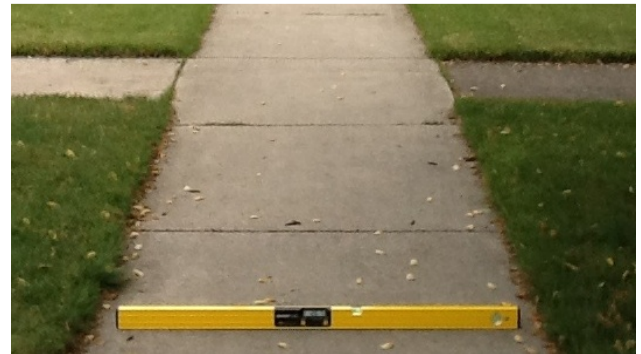
Example of Cross Slope Data Collection
